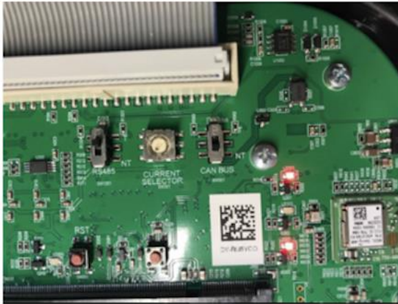
Close up RS485/ CAN bus switches
