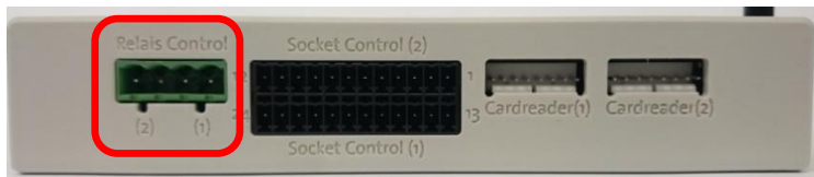
Figure 8 Charging current relay connections
