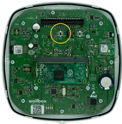
Fig. A3.1 Setting the RS485 switch to “T”
